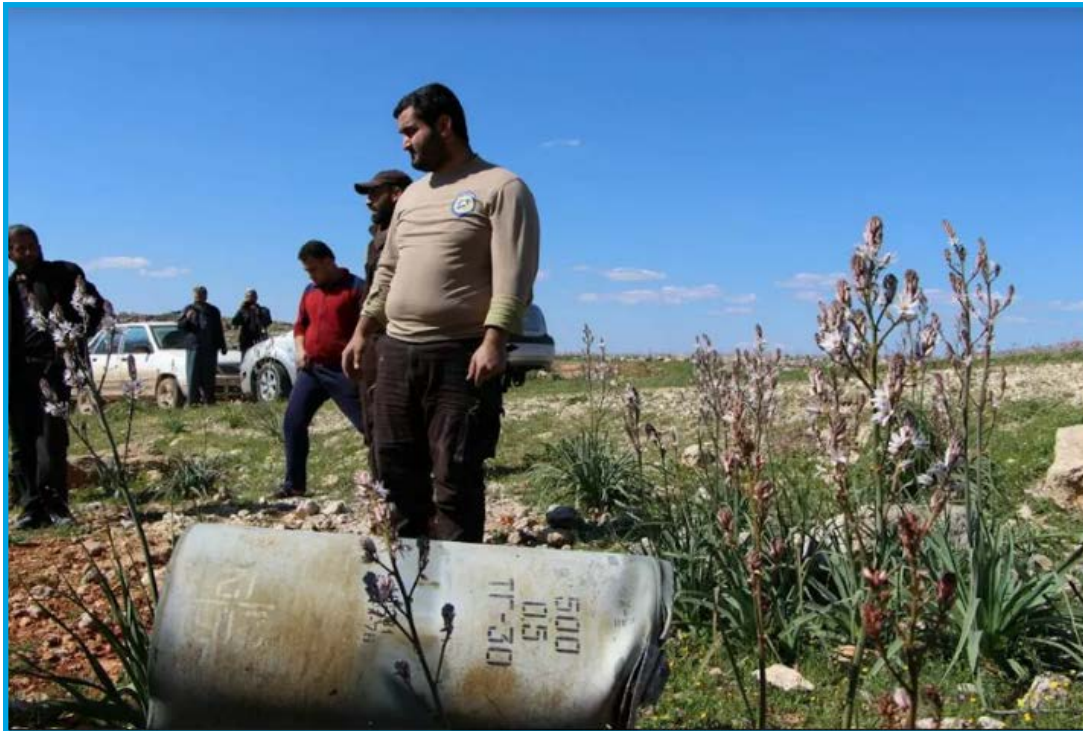
Remnants from the cover of a RBK-500 missile carrying ShOAB-0.5 submunitions found in al Tawarna village, Aleppo – March 23, 2017
